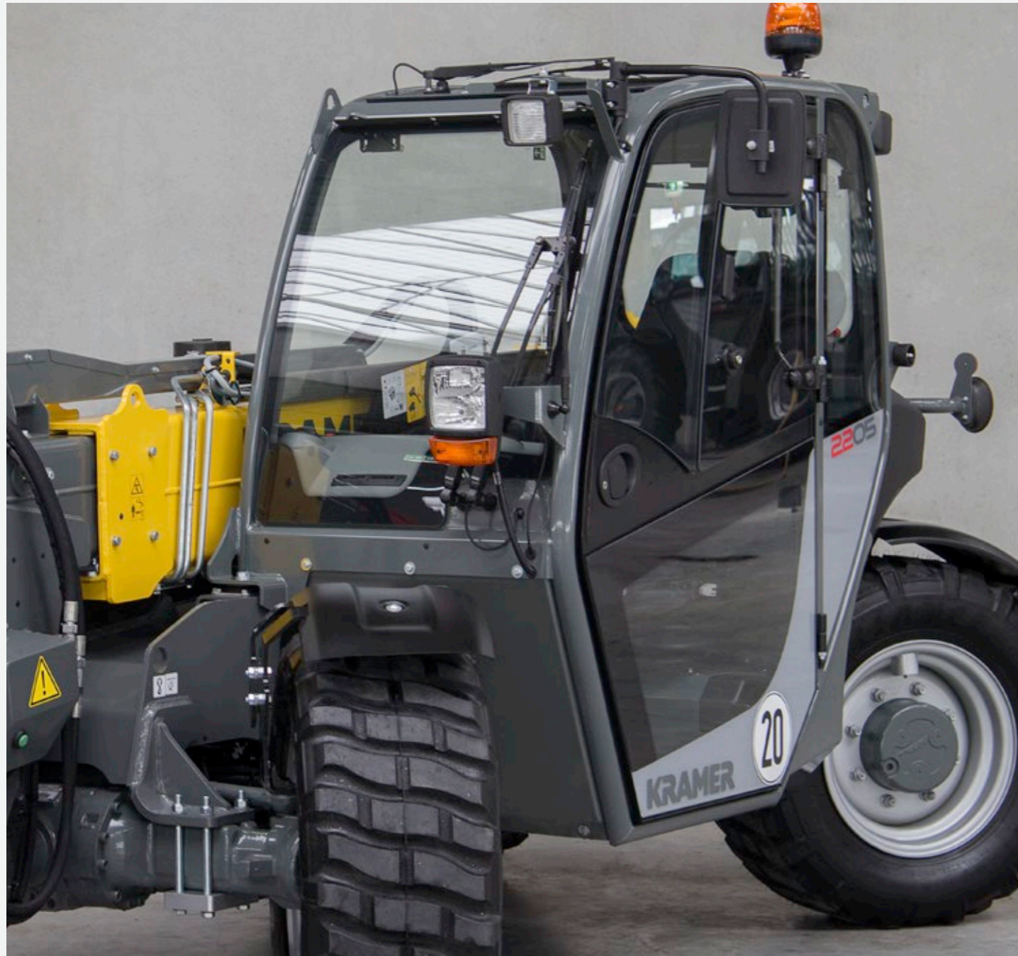
Excellent all-round visibility: Narrow cabin struts provide an optimal view on all sides.
