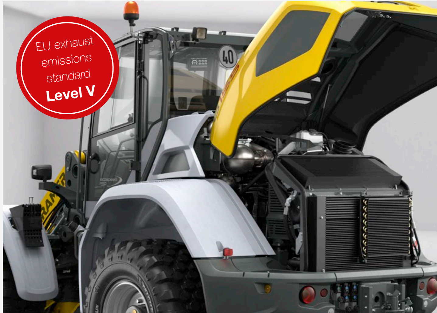
Water-cooled 4-cylinder in-line engine with cooled external exhaust gas return, turbocharging and intercooling.
