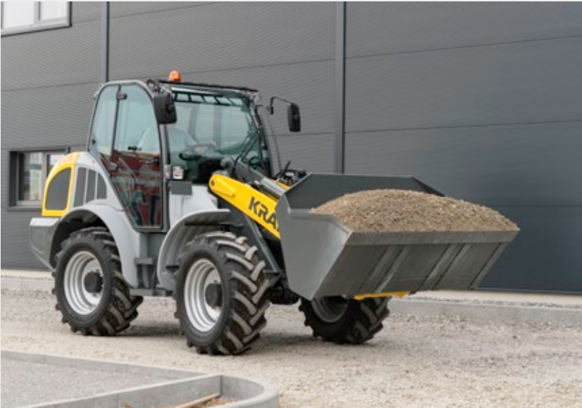
Front axle steering for increased stability during quick transport trips
