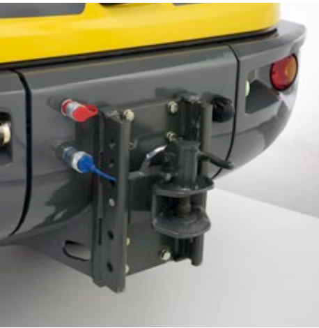
Ideal for a wide range of applications: The height of the ball hitch can be adjusted.
