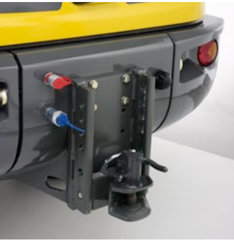
Ideal for a wide range of applications: The height of the ball hitch can be adjusted.
