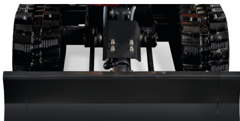
Extended undercarriage 840 mm - Increased stability
